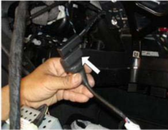
⑨ Connect the offered LCD cable to OEM cable from LCD
