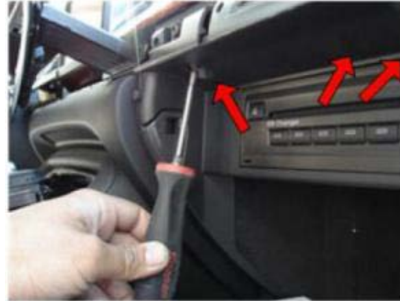
② Open Glove box after removing Screws on Dash board.
