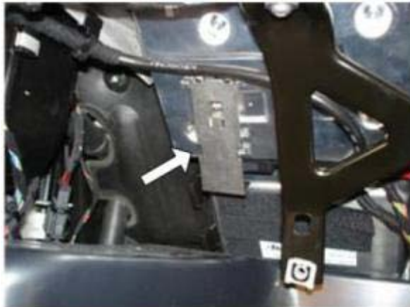
⑦ As the picture, remove the metal sleeve.
