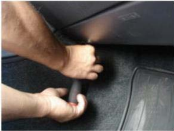
① Remove screws on Glove box.
