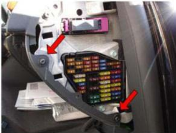
③ Open fuse box in front of passenger seat Remote swears.
