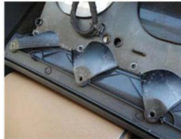
④ Pull the glove box out to take apart
