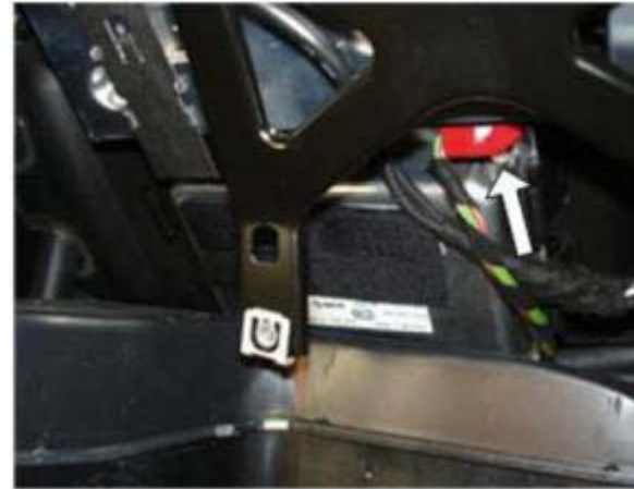
⑥ Before installation, must unplug the red original Power plug.
