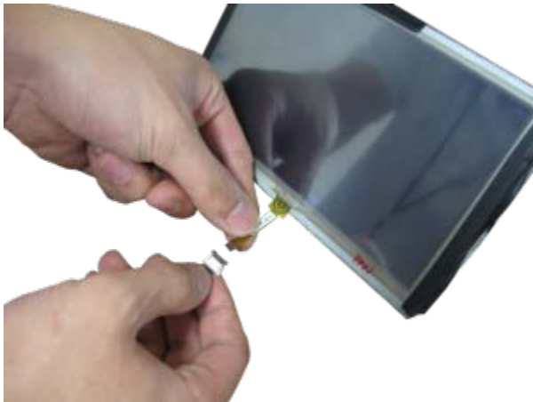
⑪ Connect Touch Out cable to Touch from LCD
